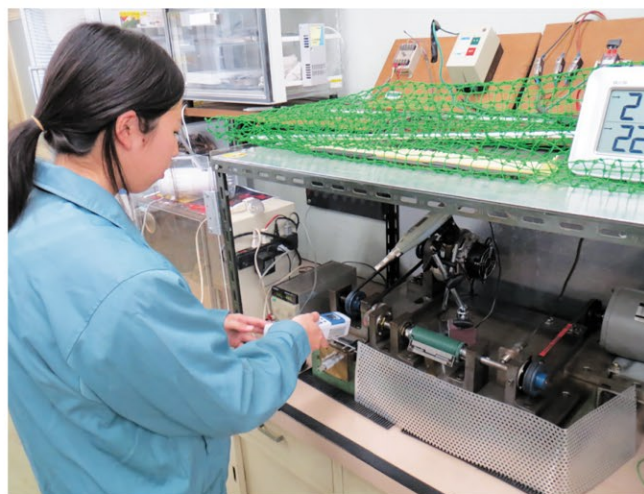
竹歯車の耐久試験 Durability Testing of Bamboo-made Gear
